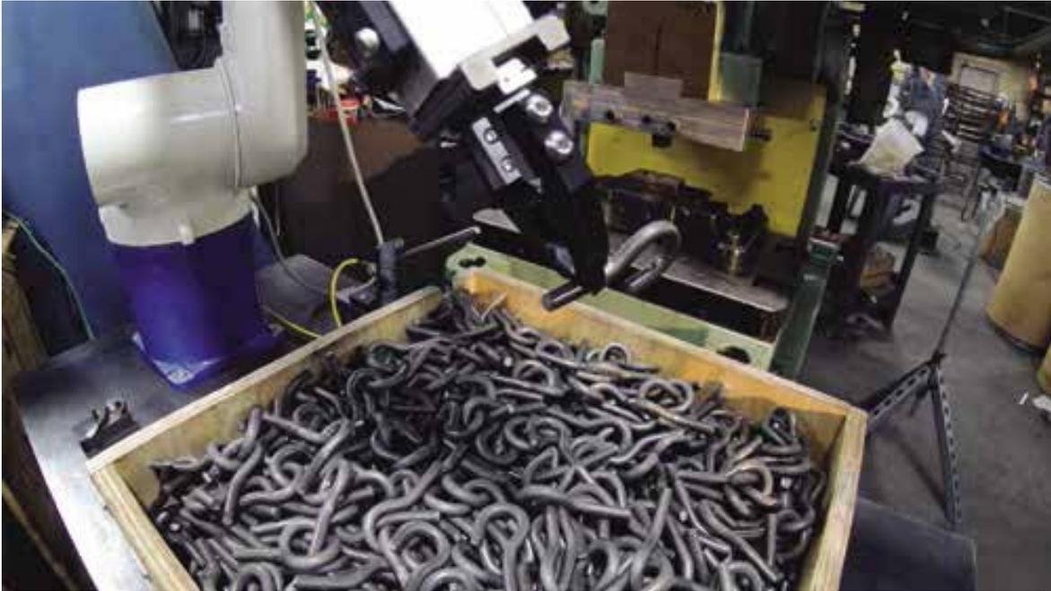
A robot at work for Ace Wire Spring. Using innovative hardware, advanced algorithms, and engineering expertise, a robot now picks hooks out of the bins and places them into a press. Photo courtesy of Ace Wire Spring & Form/CapSen Robotics.
