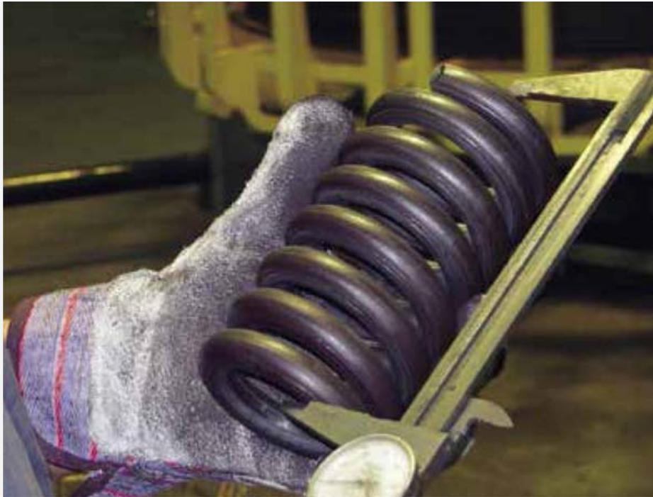
*One of Ace's coilers measures a spring to verify that its height matches the specifications. Photo courtesy of Ace Wire Spring & Form Co.*
